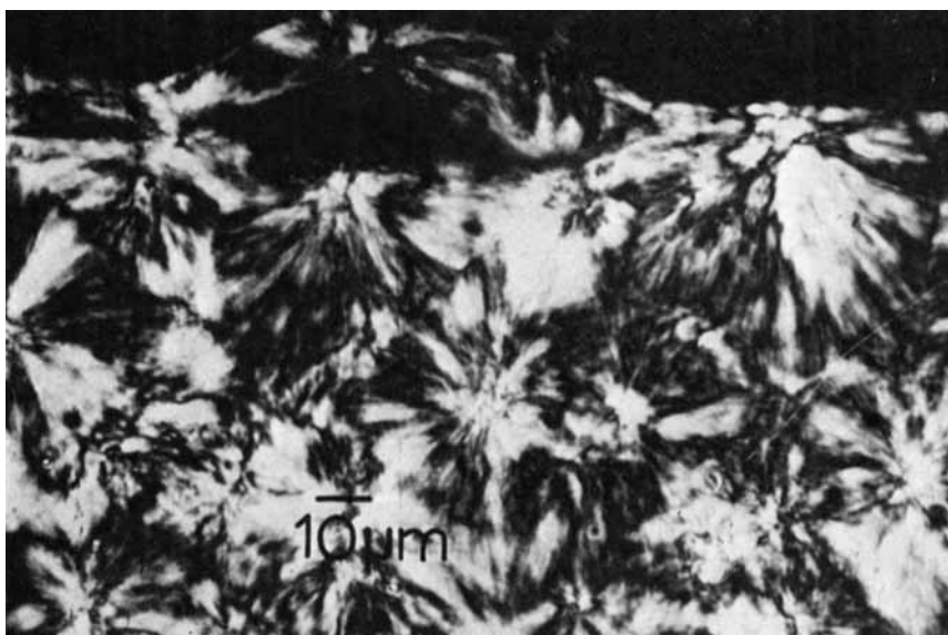
Fig. 6. Microtome section from a bulk sample of annealed-1 polypropylene treated for \frac{1}{2} hr in fuming nitric acid at 70°C. Transmitted light and crossed polars.
