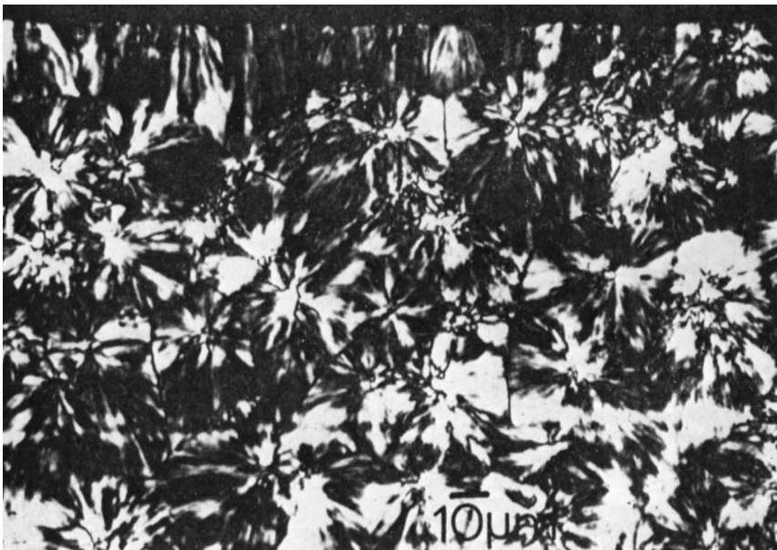
Fig. 2. Microtome section of annealed-2 polypropylene. Transmitted light and crossed polars.
