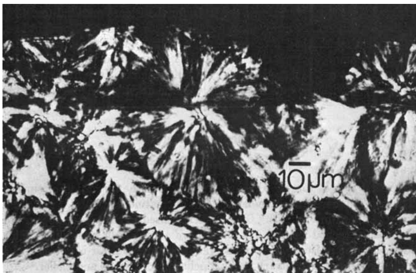
Fig. 8. Higher magnification view of the cavity in Fig. 7, showing a large crack running from center to center of neighboring spherulites. Transmitted light and crossed polars.
