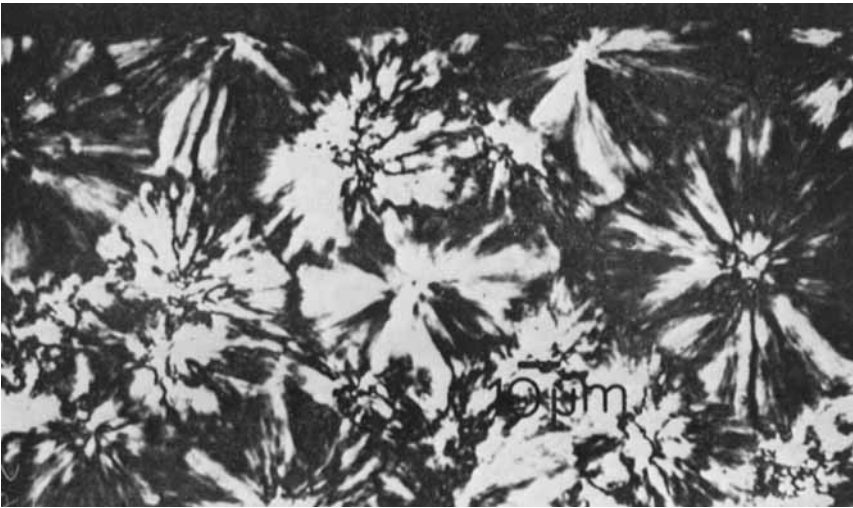
Fig. 1. Microtome section of annealed-1 polypropylene. Transmitted light and crossed polars.
