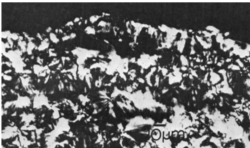
Fig. 12. Microtome section from a bulk sample of quenched polypropylene treated for \frac{1}{2} hr in fuming nitric acid at 70^{\circ}\text{C} . Transmitted light and crossed polars.
